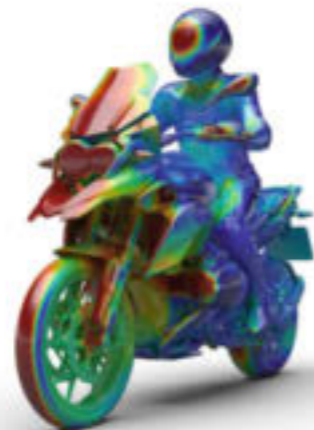
Aerodynamic simulation for visualisation of the wind-pressure distribution at the front of the helmet
